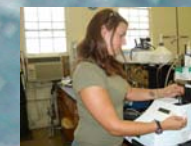
Figure 8. Using the fluorometer to measure chlorophyll concentration
