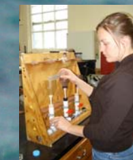
Figure 10. Filtering a water sample through a glass fiber filter.
